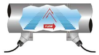
An ultrasonic meter equipped with heat flow capabilities measures the rate and quantity of heat delivered or removed from devices such as heat exchangers. By measuring the volumetric flow rate of the heat exchanger liquid, the temperature at the inlet pipe and the temperature at the outlet pipe, the energy usage can be calculated.
